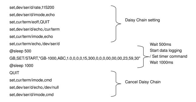
POINT: Check the Ack from Mainboard.
