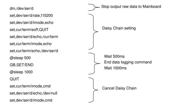
POINT: Check the Ack from Mainboard.
